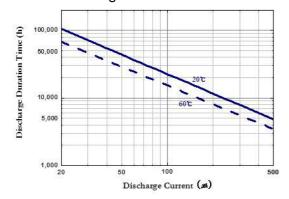
This data was made on basis of nominal capacity for the purpose of enabling users to forecast approximate life time. In order to calculate precise life time under various environments, we recommend you to consult VARTA Microbattery GmbH. In case where the products are improved, the specifications described herein are subject to change.
